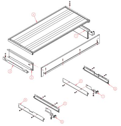
4. Arion Aisle Containment Top Panel standard 600W/800W
