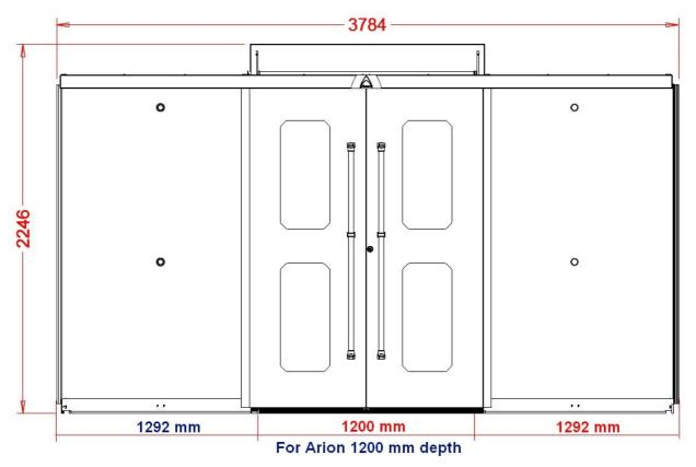
Dimension for Arion Cold Aisle containment 600W/800W 42U 1200 mm depth.
